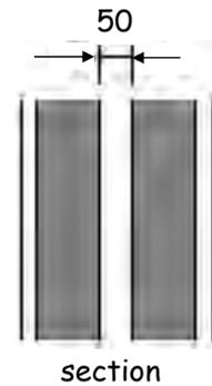
Wall type 2C Two leaves of concrete block with 50 mm cavity, both leaves parged, gypsum based board on both *room* faces.
