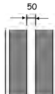
Wall type 2B Two leaves of concrete block with 50 mm cavity, plastered on both *room* faces
